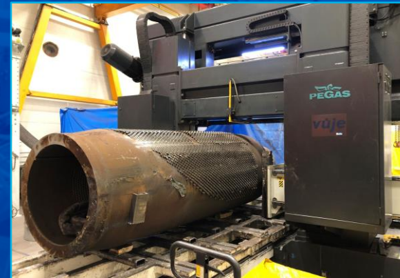
SG collectors fragmented by band saw
