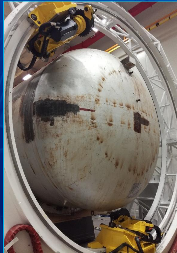
SG shell cutting device
